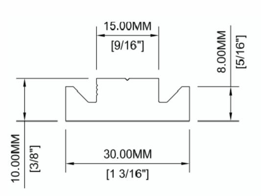
These drawings are published as an information guide only. These CAD drawings are intended as templates to assist the designer, they do not contain the full detail required for construction and must be read in conjunction with the installation instructions on www.facadespecialtiesinc.com. You should obtain architectural, engineering or other technical advice to assess the suitability of these drawings to the requirements of your particular project.
