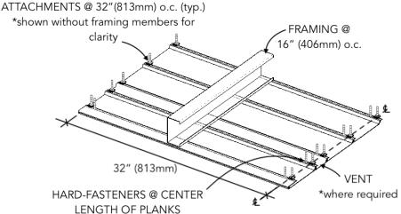
If installing with staggered butt-joints, hard-fasten the two planks at the butt-joint to ensure joints do not open up (see Detail A&B). Fasteners should be anchored into a solid secure framing member, blocking, furring strip or backer plate\* etc. (\*see Detail B). Use touch-up paint pens (purchased separately) to finish the ends of the two (2) planks at the butt-joint.
