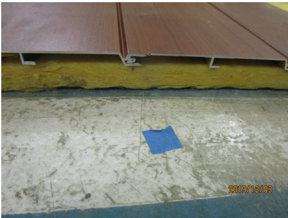
Figure 2 – Detail of tongue and groove joints, fiberglass backer
