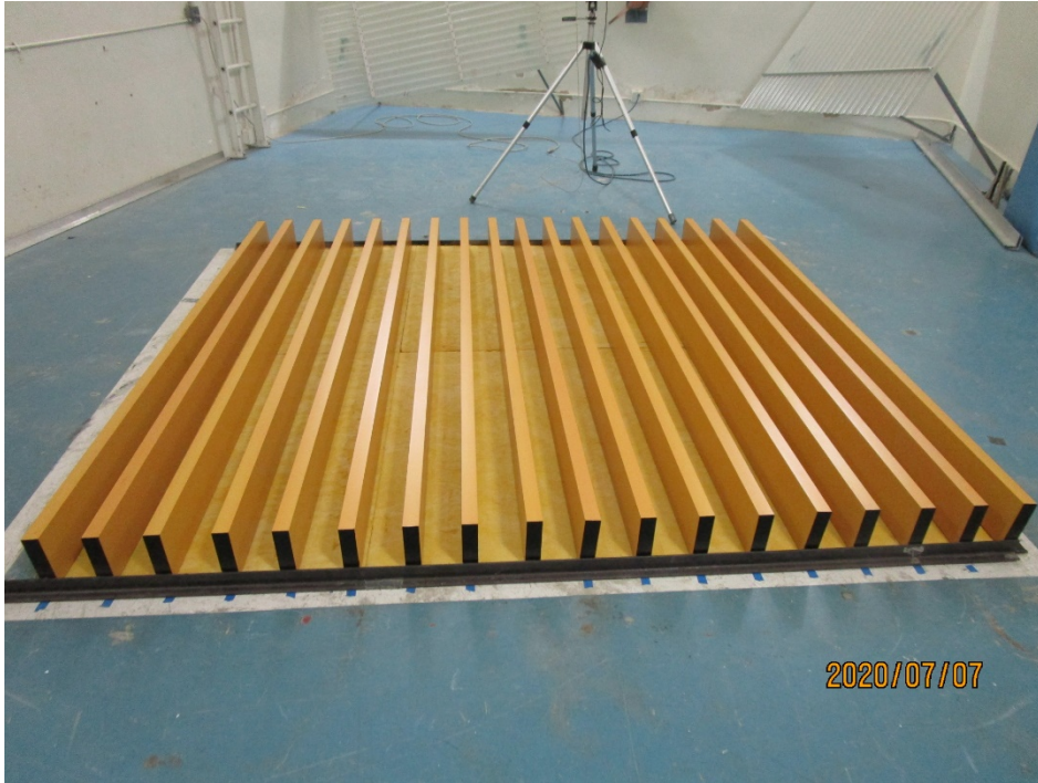
Figure 3 – Specimen mounted in test chamber
